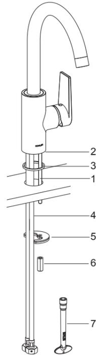
Install the mounting stud(1) into the faucet body base(2). Insert the washer (3) under the body assembly. Insert the flexible supply hoses(4) into the sink.
