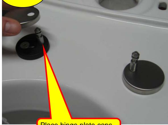
Place hinge plate caps onto hinge plates
